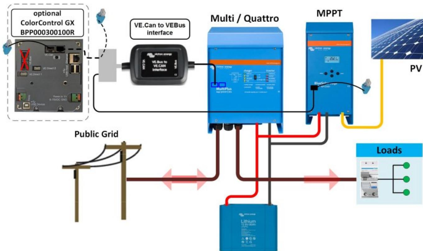
Either way, with or without CCGX, make sure that the VE.Can network is terminated on both sides, using the VE.Can terminators supplied with the CCGX and the MPPT charger controllers. They are also available for purchase as a [separate accessory](#).
