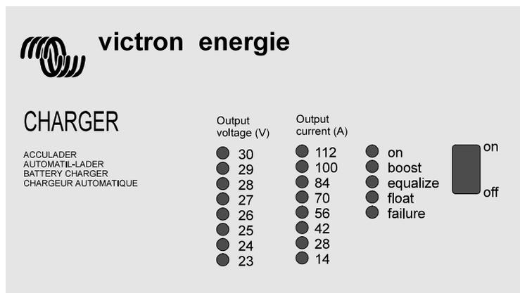
Illustration 5. Example of the battery charger front panel.
