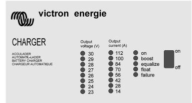
Illustration 5. Example of the battery charger front panel.
