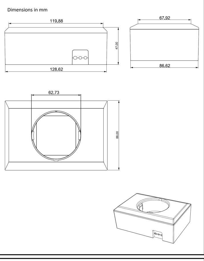
Dimensions of ASS050500000 Box for Wall Mounting of BMV battery monitor
