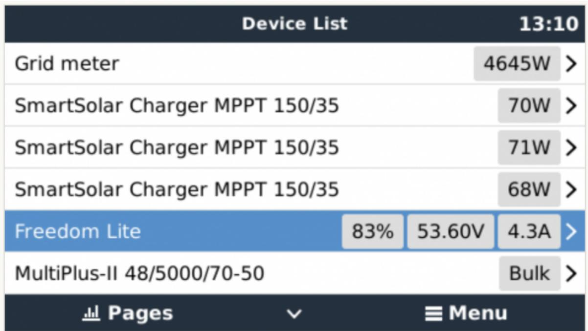
Freedom Won LiTE → Parameters → Confirm that the Charge Current Limit and Discharge Current Limit are as per the LiTE specifications.
